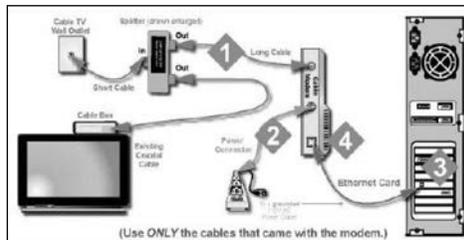
Figure 2.3: Typical Ethernet cable modem installation
